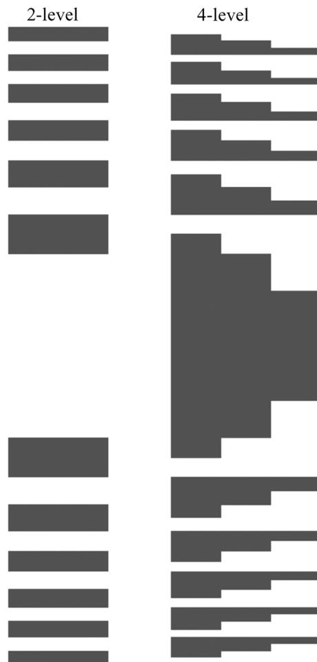
**Fig. 9** Two-level phase type Fresnel zone plate (FZP) with 40% efficiency (left), Four-level phase type FZP with 81% efficiency (right), which needs two additional electron beam lithography (EBL)/etching mask deposition/anisotropic etching steps. Adopted from Ref. 15
