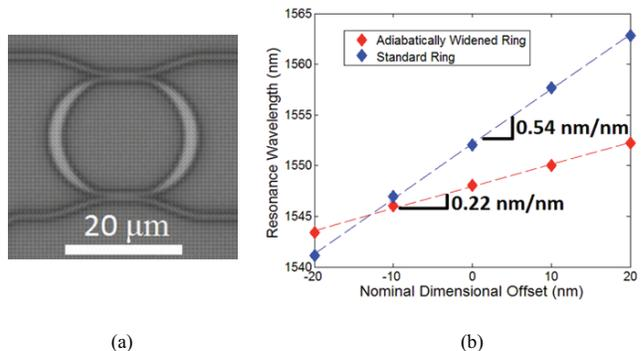
Fig. 1. (a) Optical microscope image of a fabricated adiabatically widened microring in SOI with an oxide cladding. (b) Resonance wavelength shift as a function of the nominal dimensional offset. (From [6])
