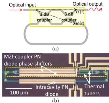
Fig. 2. (a) Schematic of a coupling modulated microring. The box marks the  $2 \times 2$  MZI-coupler. (b) The fabricated SOI MZI-microring. (From [13])
