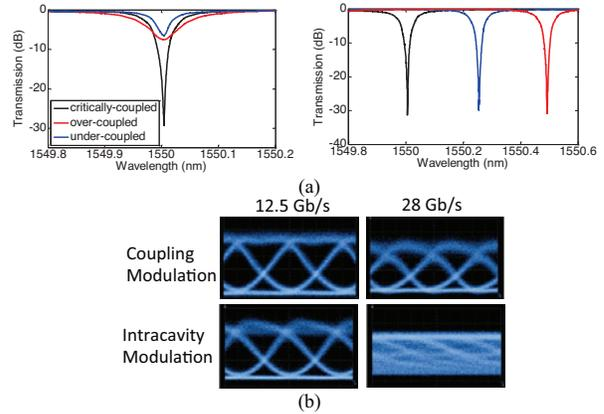
Fig. 3. (a) Measured transmission spectra as the coupling coefficient is tuned at a fixed resonance (left) and as the resonance wavelength is tuned with a fixed coupling coefficient (right). (b) Eye diagrams for coupling and intracavity modulation at 12.5 Gb/s and 28 Gb/s. (From [13])
